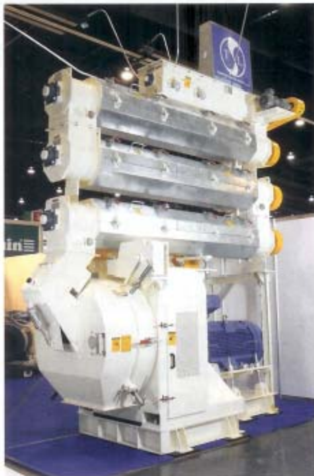
The TEC pelleting mill evolved from a simple tapioca mill to a professional pellet mill for animal feeds.
